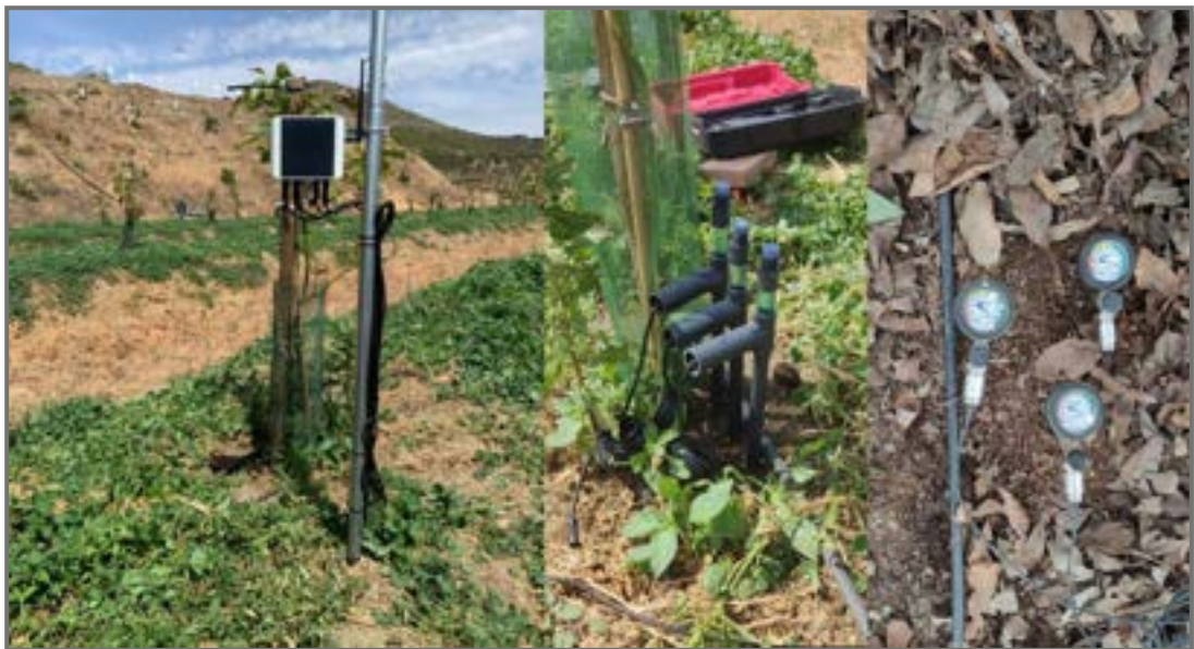
Tensiometers are used to monitor soil moisture and are incorporated into irrigation systems. Photos supplied by TROPS
